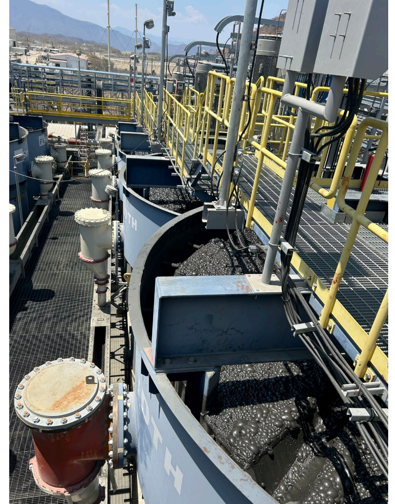
Cu and FeS flotation circuit
