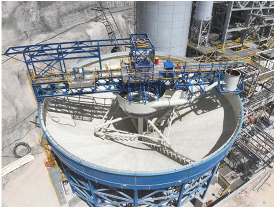
Figure 4: Paste plant thickener ready for water testing.
