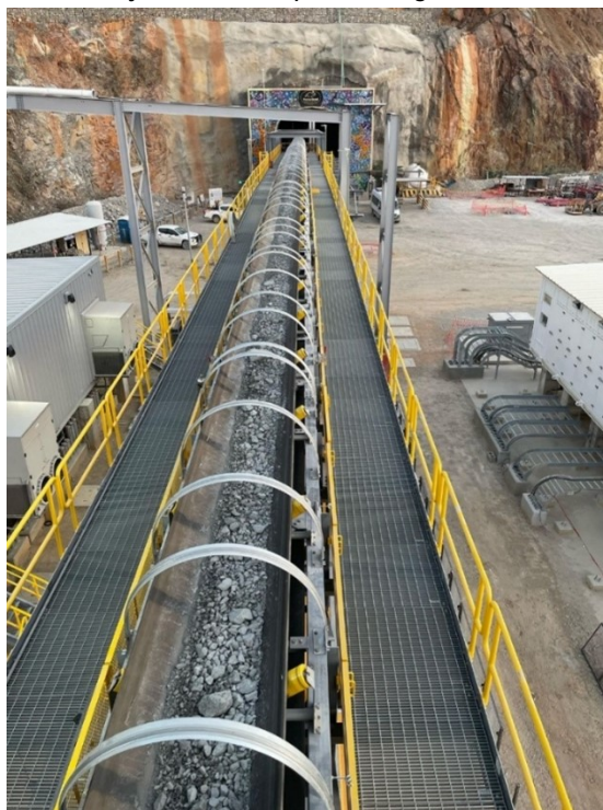
Figure 1: Commissioning of the Guajes Tunnel conveyor was completed during the quarter. Ore is being transported through the tunnel out of the Guajes Portal for processing on the north side of the Balsas River.
