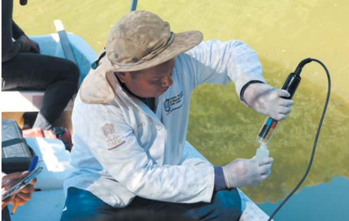
UAGro Field Technician preparing a water sample for laboratory analysis on the Río Balsas (July 2025)
