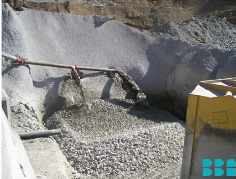
Figure 16-61: Mixing Pit Example
