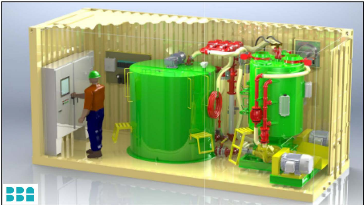
Figure 16-60: Portal 3 Slurry Mixing Unit
