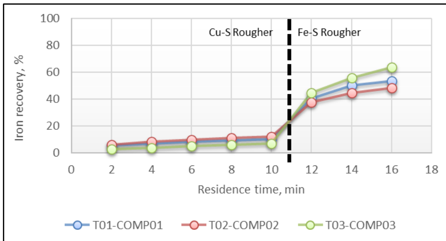
Figure 13-44: FS-MLL Evaluation of Iron Flotation Kinetics in the Copper and Fe-S Rougher Stages
