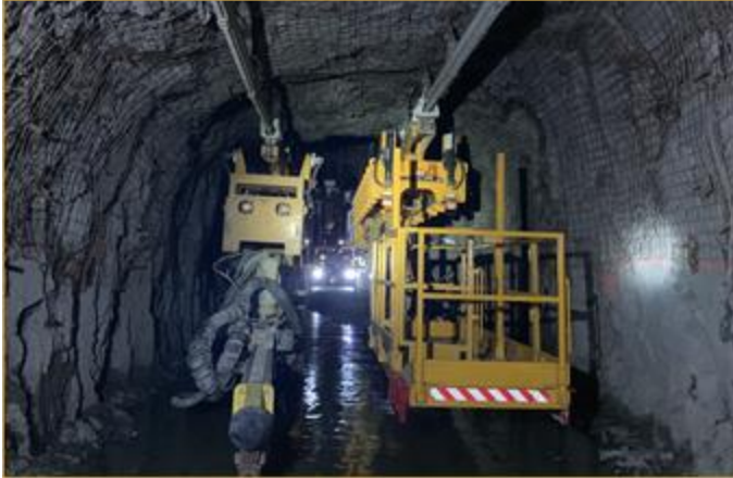
Two-way traffic via dual monorails
