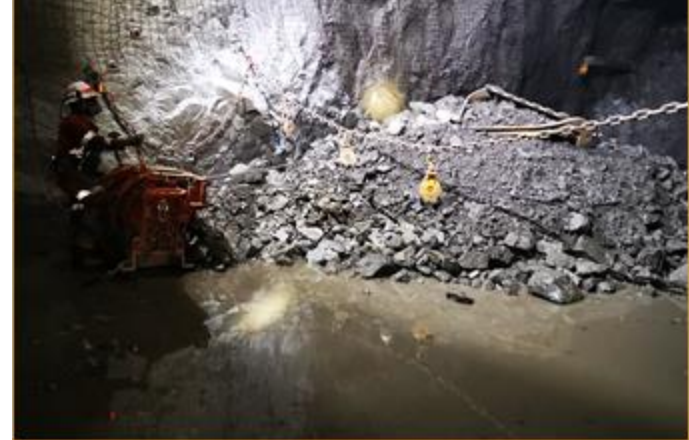
Mucking out a stope with a slusher
