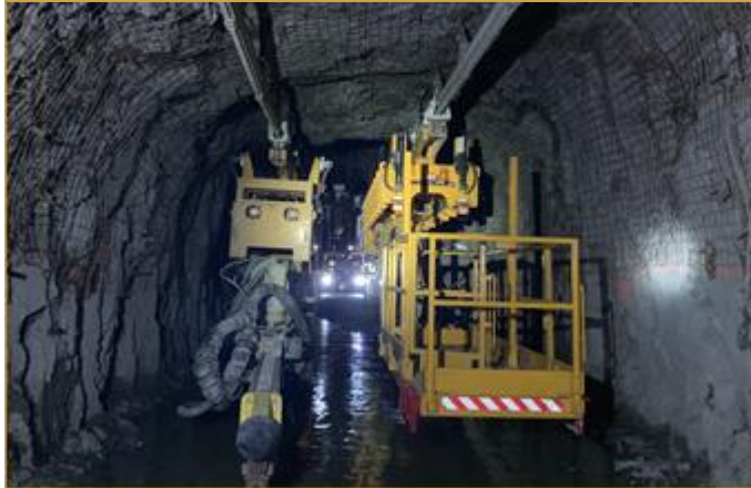
Two-way traffic via dual monorails
