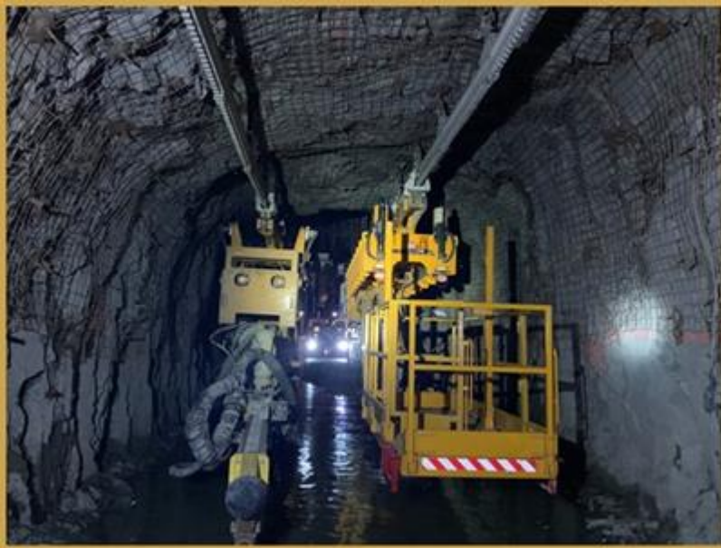
2-way traffic flow made possible by dual monorails hung off the back.
