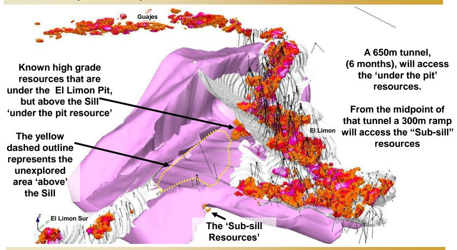
...the tunnel will provide access to targets above & below the Sill
