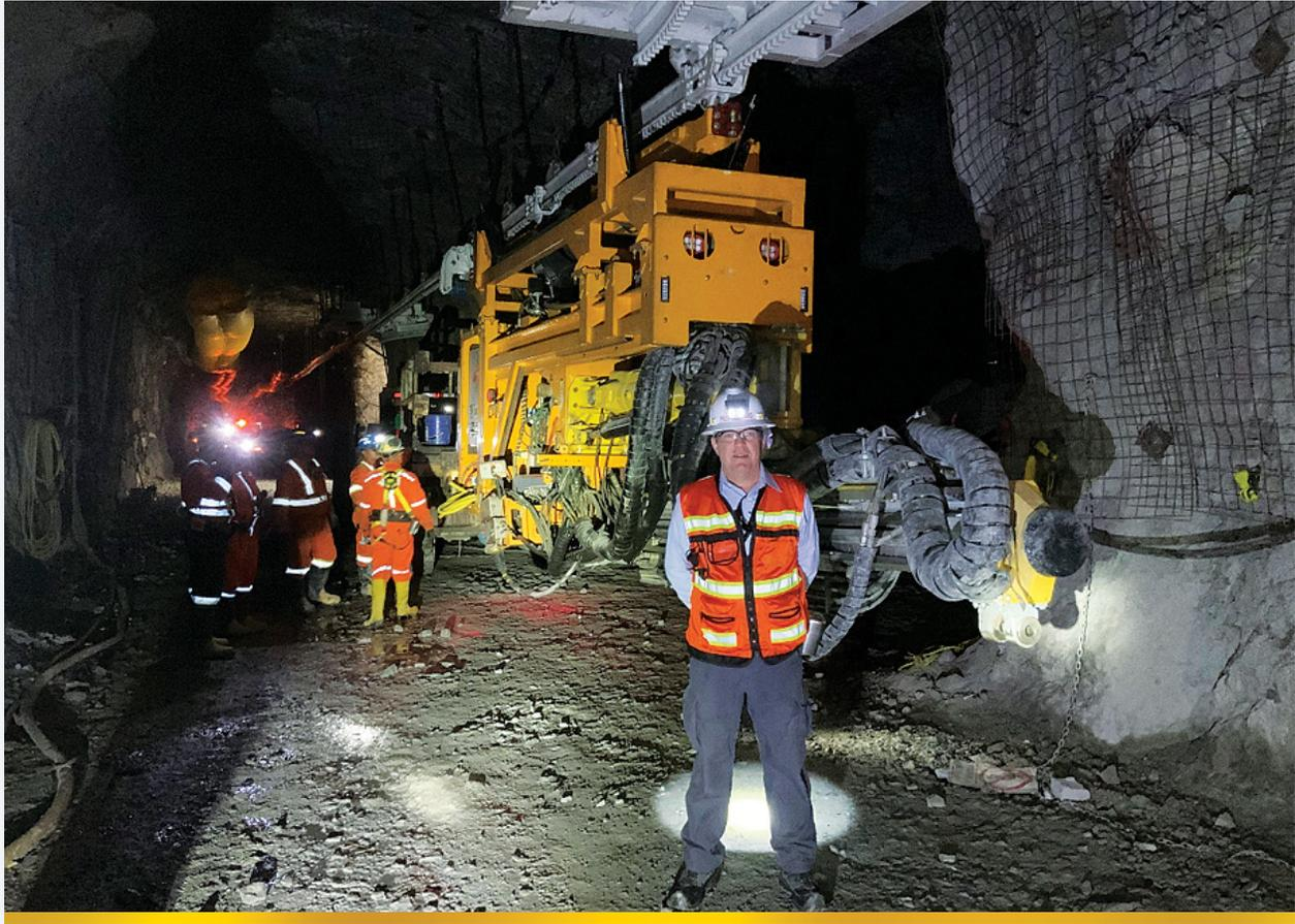
Another great example of our innovative approach to mining is the Muckahi mining system – a Torrex innovation – which has been in test use in the El Limón Deep underground mine since early 2019.
